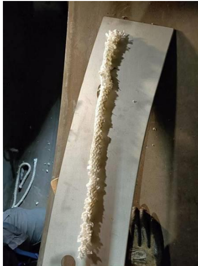
Figure 11: Discarded rope seal shell
