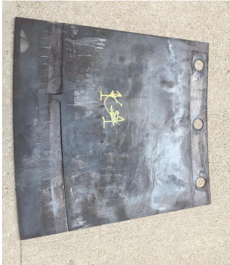
Figure 4. Flex seal wear due to sharp edges on flex seal clamp plates
